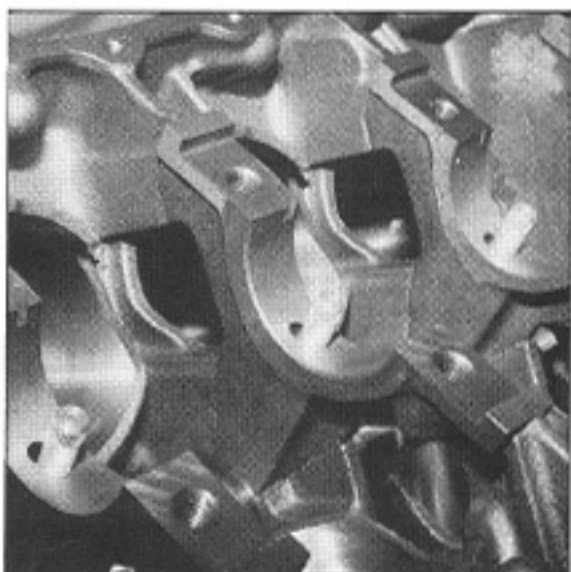
The nodular iron 350 Olds crankshaft is easily identified by the large "N" at the front. Notice the ST950 main cap strap and bolts in place.
