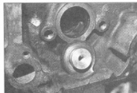
Number 1080 aluminum plug is used to block off the injector drive oil hole when using the diesel cam bearings. The center is threaded for easy installation using a common head bolt.
