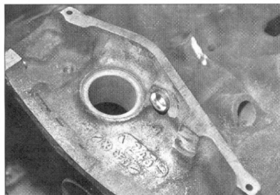
This is where the factory injector oil drain hole is located. It can be blocked with an 11/16th cup plug, as shown here.
